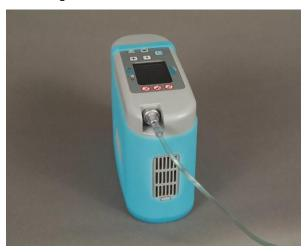
6. Turn on the Nano by quickly pressing the ON/OFF button (§4.3). The indicator light will flash and the display will show the Nidek Medical Products, Inc. logo upon startup.
